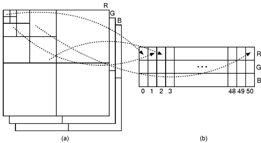
**Fig. 2.** Procedure used to construct a chromosome. (a) Wavelet transformed  $256 \times 256$  images. (b) The chromosome constructed using the wavelet coefficients of (a).
