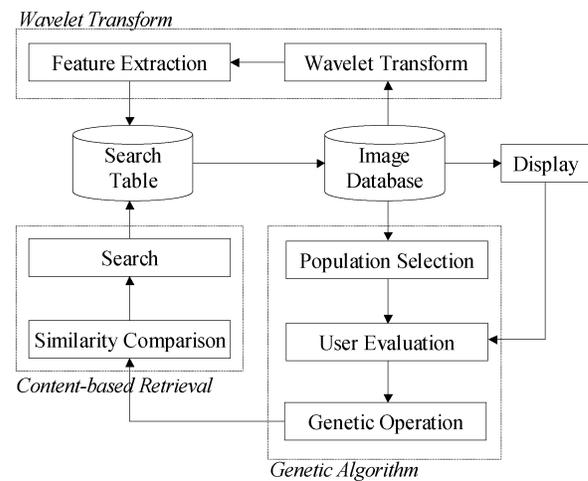
Fig. 1. Image retrieval system using IGA.
