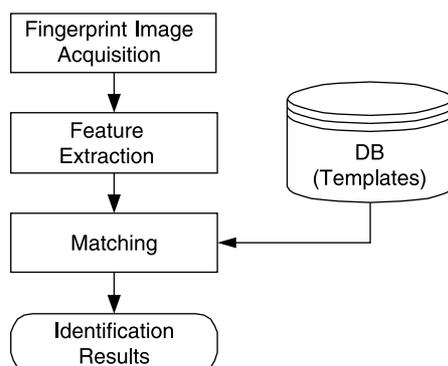
Fig. 2. Architecture of a fingerprint identification system.
