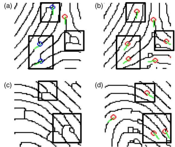
Fig. 14. Oily image examples of minutiae extraction with conventional/adaptive filtering: (a) and (c) show the extracted minutiae with the conventional filtering, (b) and (d) show the extracted minutiae with valley enhancement.
