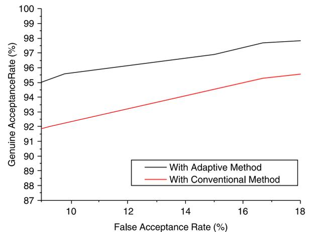
Fig. 15. ROC curve comparing the performance of the proposed method with the conventional method.
