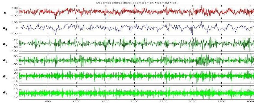
Fig. 1. Discrete wavelet transforms of a sample EEG signal using DB2 and decomposed up to level 4
