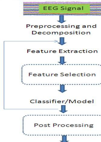
Fig. 2. Process of EEG Signal Analysis
