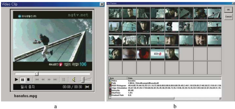
Fig. 6 Interface for examining a video: a the way of seeing the whole frame sequence (by pressing the ► button under key frame image) b the way of seeing only key frames (by pressing (i) under key frame image)
