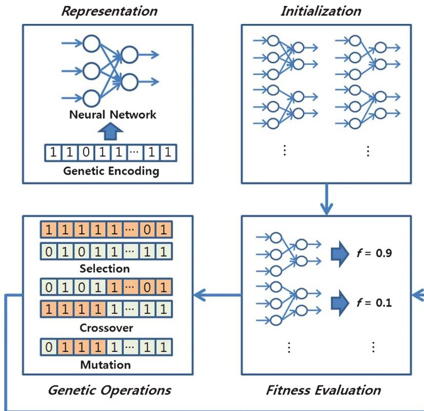
Fig. 1. Overview of the evolutionary neural network algorithm.
