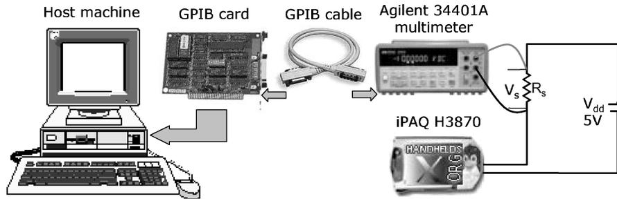
Fig. 10. Power measurement setup.
