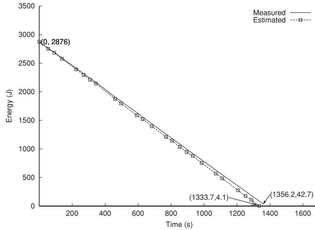
(c) Comparison of estimated and measured energy-dissipation rates
